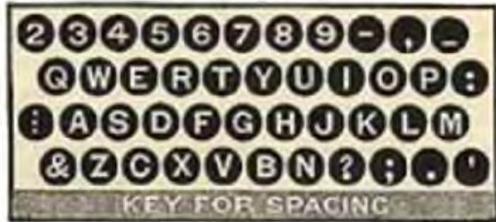
Sholes & Glidden's 1873 Keyboard Arrangement
